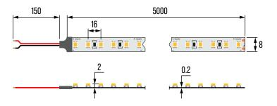
Unit: mm Cut: 49.21mm -Connection diagram
