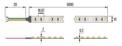
Unit: mm Cut: 100mm -Connection diagram
