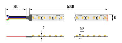
Unit: mm Cut: 100mm LED type: 2835 RGB -Connection diagram
