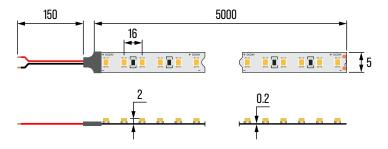
Unit: mm Cut: 100mm -Connection diagram
