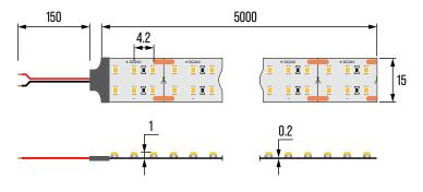
Unit: mm Cut: 12.7mm -Connection diagram
