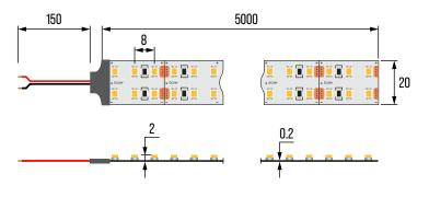
Unit: mm Cut: 49.21mm -Connection diagram
