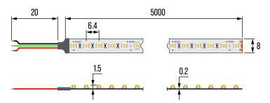
Unit: mm Cut: 38.1mm -Connection diagram
