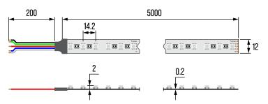
Unit: mm Cut: 82.55mm LED type: 5050 RGBW -Connection diagram
