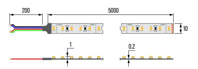
Unit: mm Cut: 49.21mm LED type: 2835 RGB -Connection diagram
