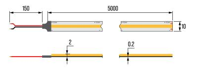
Unit: mm Cut: 38.46mm -Connection diagram
